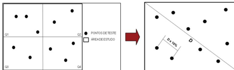
**Figure 3:** Example of point distribution inside the grid and according to a minimum distance.
