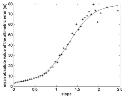
Figure 2: mean absolute value of  $\varepsilon_{\text{DEM}}$  as a function of the DEM slope
