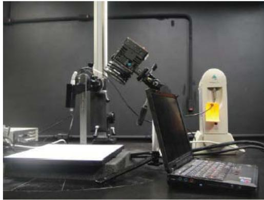
**Figure 3:** Overview of the experimental setup to obtain the reflectance factor of the reference panels.
