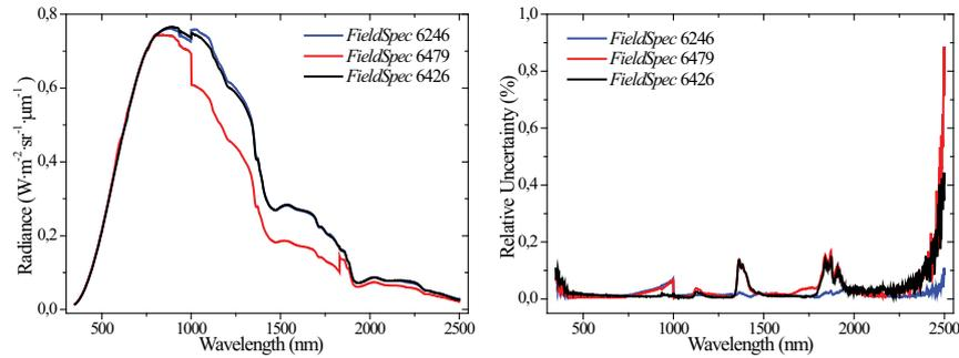
**Figure 4:** In (a) the radiance plot as a function of wavelength, with the three spectroradiometers with 25° FOV. Measurements were taken with the lamps 150, 100 and 45 W of IS turned on (total power of 295 W); in (b) graph of uncertainties as a function of wavelength, obtained with each of spectroradiometers.
