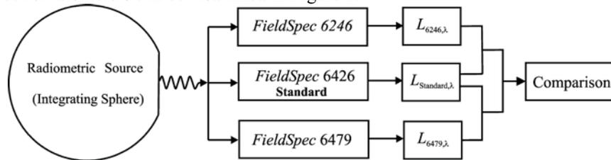
**Figure 1:** Flowchart of the methodology to calibrate the two spectroradiometers used in the fieldwork.
