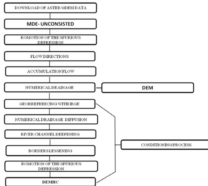
Fig. 2: Diagram representing treatment and conditioning procedures of DEM
